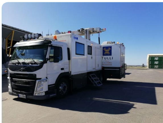
Vehicle scanner purchased by Finnish customs through the Hercule Programme managed by OLAF
